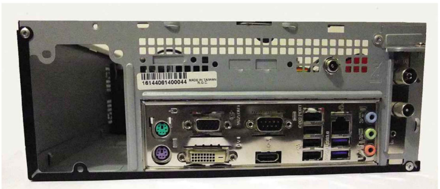
▲ The rear of the case. There was a convenient punchout to fit the 12V input for the PSU just above the I/O shield
