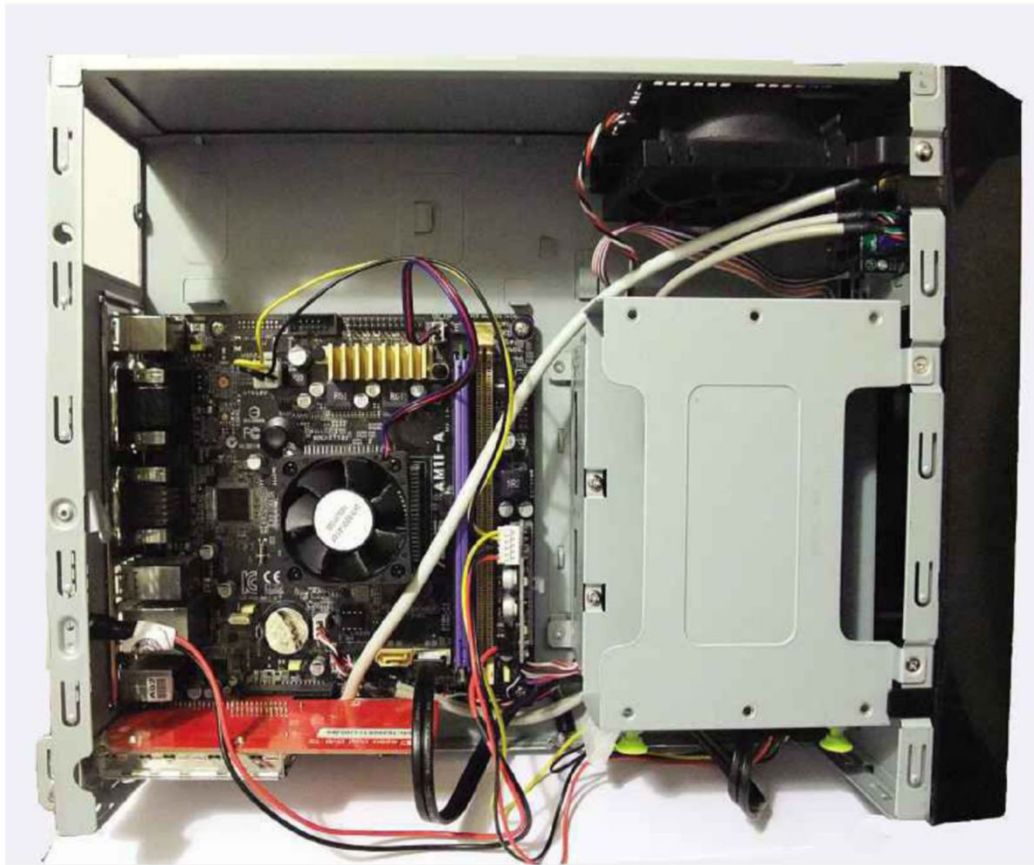
◀ Inside the Case, with the motherboard in place and the PicoPSU connected. The large space at the top of the picture is where the original PSU was sited
